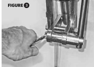
**3 INSTALL** the lever clamp. When sliding the lever through the lever clamp, make sure the lever passes all the way through the lever sleeve [FIGURE 3] to prevent breakage. The lever angle is adjustable by loosening the lever clamp bolt just enough to allow the teeth on the lever sleeve and toggle link to slip past one another and the lever can be installed on either side of the press for right or left handed operation.
