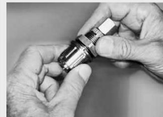
Thread your die into a quick-change holder and lightly snug the lock ring
