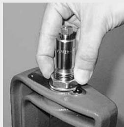
Notice how the lock pin is automatically depressed, allowing instant one-handed removal.
