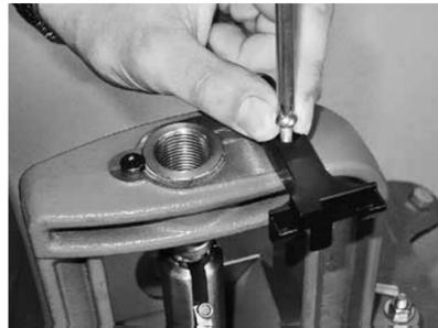
**1** INSTALL primer feed bracket with supplied 10–24 screws.
