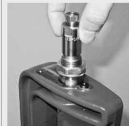
Insert the holder into the press so that the lock groove will line up when secured. Adjust your die in or out for proper operation.
