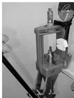
8 LOWER ram (raise handle) to seat the primers. The primers should be flush to slightly below flush when properly seated.
