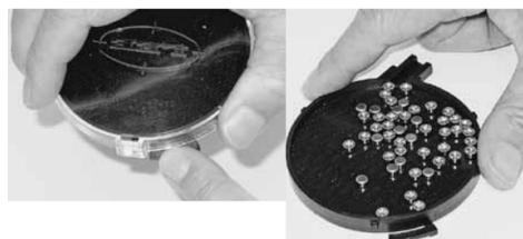
**4** DEPRESS primer latch on tray, rotate counterclockwise and lift off cover. Place no more than 100 primers in tray; shake side to side to tip primers upright.
