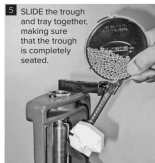
5 SLIDE the trough and tray together, making sure that the trough is completely seated.
