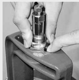
Remove the die by depressing the lock pin; rotate die 1/6 of a turn. Lift out and change to your next die. After your dies are set, they can be installed so that the lock groove does not line up with the lock button.
