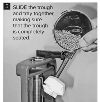
**5** SLIDE the trough and tray together, making sure that the trough is completely seated.
